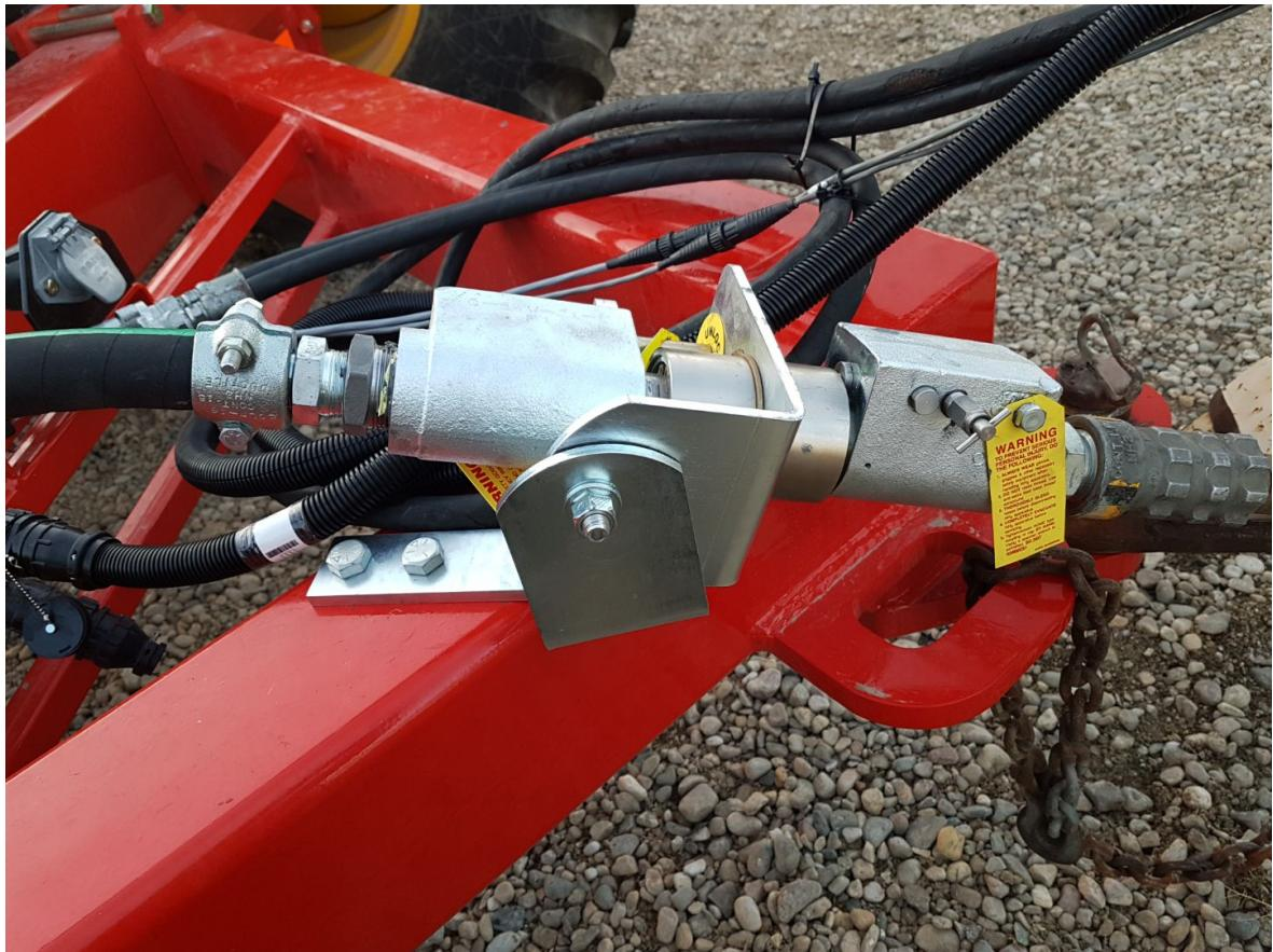
2. Most applicators will have a bracket available to fasten the breakaway too. Follow the manufacturer's recommendations when mounting the breakaway and hose couplers.
