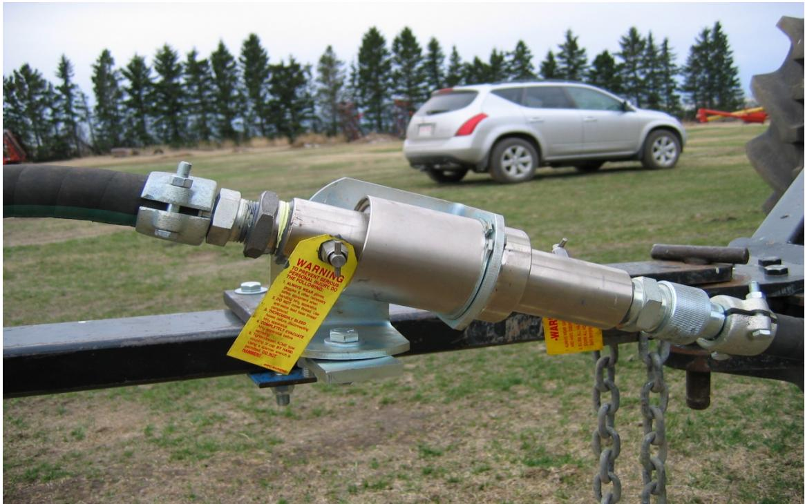
5. Install the breakaway that is in front of the air cart(TBH only). Install the male tip on the air cart side of the hitch and the female coupler on the air drill side of the hitch.
