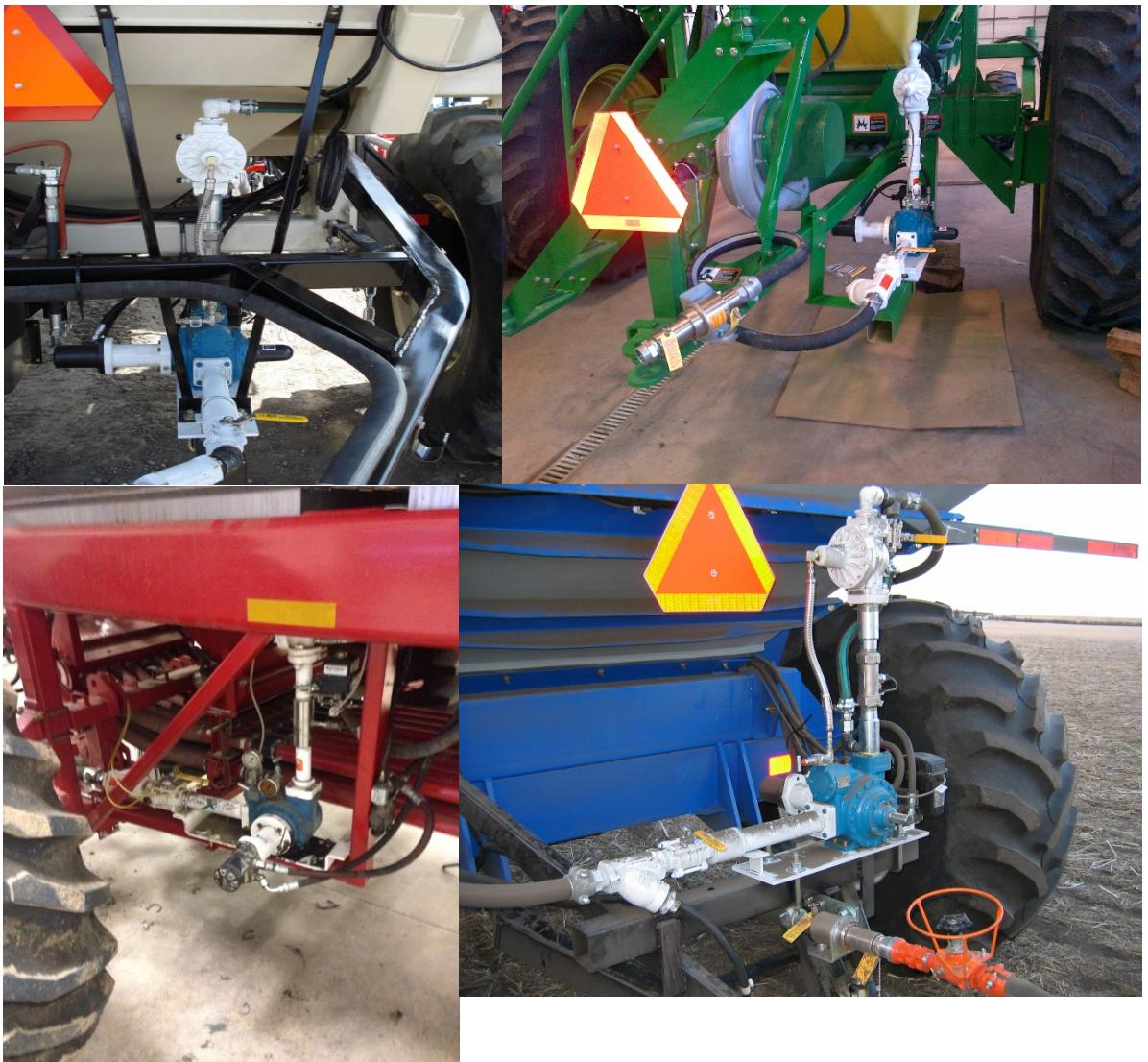
When mounting pump on applicator or the back of the air tank in a tow behind air tank configuration;
